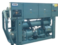
YLCS Water to water HP Twin screw / R134a (R513A on request) Hot water up to 65°C Heating capacity: 469 to 1300 kW
