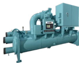
YK Water to water heat pump VSD Centrifugal compressor R513A Hot water up to 50°C Heat. cap.: 1000 to 9000 kW
