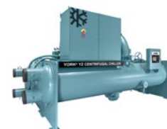
YZ Water to water HP VSD Centrifugal compr. Mag. bearings R1233zd(E) Hot water up to 45°C Heating capacity: 1000 to 6800 kW
