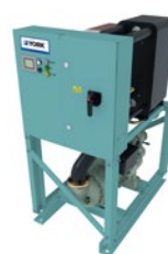
YCSE HP Water to water HP Screw compr. / R134a (R513A on request) Hot water up to 50°C Heating capacity: 170 to 300 kW
