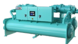
YVWH High Head HP Water to water HP VSD Screw compr./ R1234ze Hot water up to 80°C Heating capacity: 800 to 1600 kW
