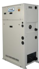
YMWA Water to water HP Scroll compr. / R410A Hot water up to 55°C Heating capacity: 24 to 215 kW
