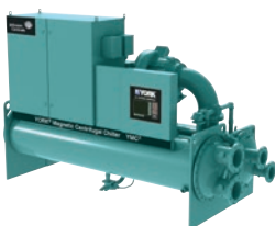
YMC 2 Water to water heat pump VSD Centrifugal compressor, Magnetic bearings / R513A Hot water up to 65°C Heat. cap.: 1600 to 3000 kW
